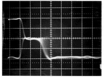
Metastability. The output of a flip-flop sits halfway between 1 and 0
