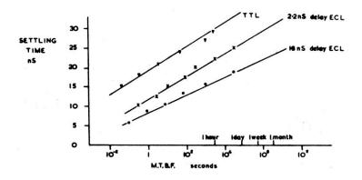
Waiting time against mean time between failures
